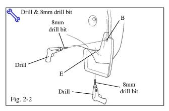
(c) Hold the part up and into bumper to use it as a template. Drill 8mm holes in locations B and E (Fig. 2-2).
